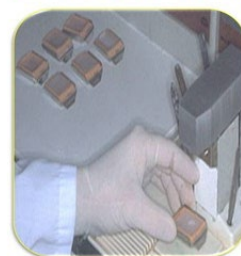
Add cassette, fill with wax and put on cold plate
