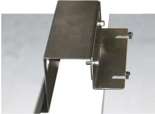
Figure 5. Autoslide cart bracket with loosened screws
